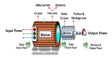
A three-phase induction motor is the most commonly used AC motor in industries due to its ruggedness, low cost, and self-starting feature. It works on the principle of electromagnetic induction.
